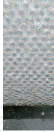
Autogenous wear protection: ground material accumulates between the hard metal studs and thus minimises roll surface wear.
