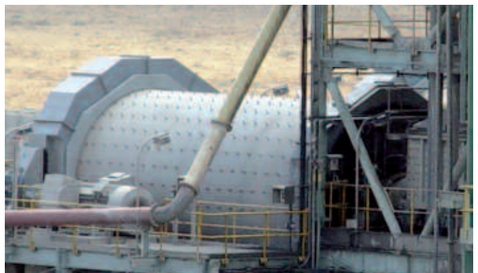
POLYCOM® and scrubber from Polysius: core process technological components of a diamond ore processing plant.
