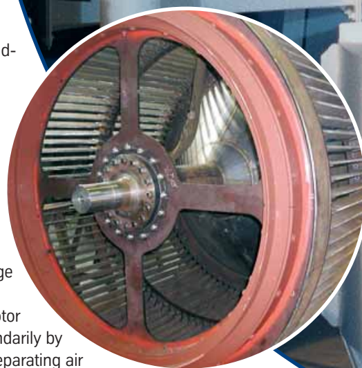
Assembled separator cage of a SEPOL®-SV high-efficiency separator.
