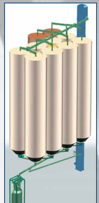
The individual cells of the multi-cell silo are filled one after the other but emptied simultaneously.
