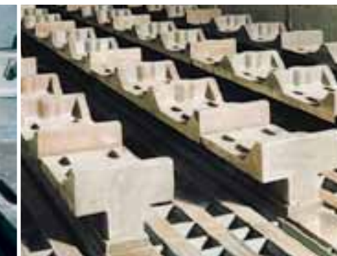
The clinker is transported by the synchronised forward movement of all the transport tracks.
