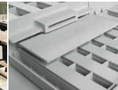
The air blast units installed between the grate steps of the static primary grate enable highly-effective elimination of snowman at the specific points where they form.
