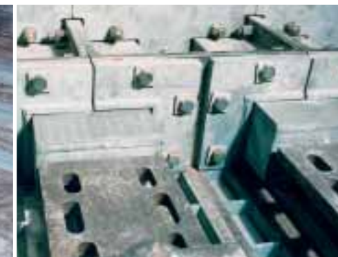
Specially developed low-wear sliding elements reliably seal the few contact zones between the static and the moving cooler components.
