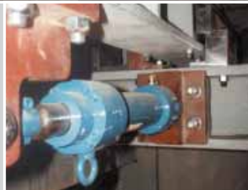
New, unconventional solutions provide the basis for the sophisticated clinker transport mechanism: the transport tracks are driven by hydraulic cylinders installed underneath the static aeration floor.
