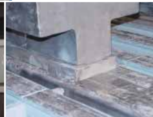
New, unconventional solutions provide the basis for the sophisticated clinker transport mechanism: the transport tracks are driven by hydraulic cylinders installed underneath the static aeration floor.
