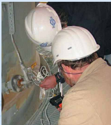
Obtaining of samples for gas analysis and dust measurement with a water-cooled probe.
