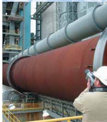
Measurement with the thermo camera for determining heat losses.
