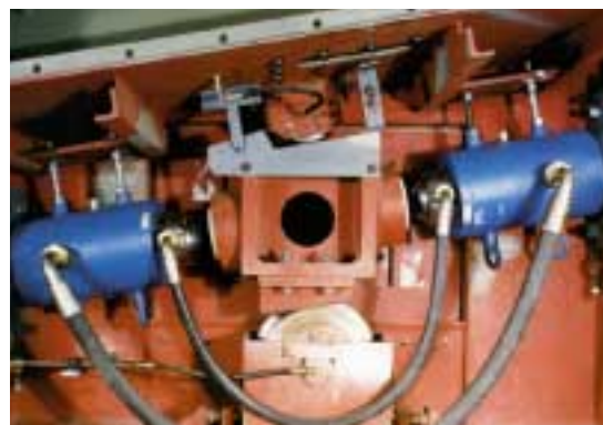
Hydraulic drive unit of a clinker grate.
