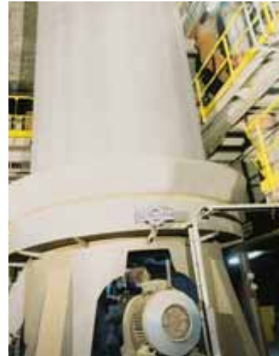
Drive unit of the fines cooler.
